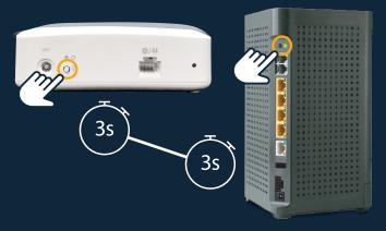
**Note:** Once successful pairing is complete, the GigaSpire Router and Wi-Fi Extender LEDs will both show a solid green color. It may take several minutes to reach this state.
